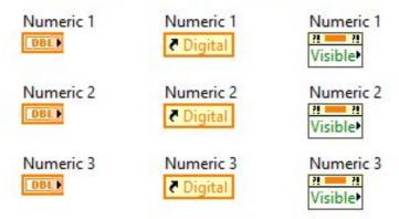
Whoa there pardner, not so fast. The control reference labeled "Numeric 1" is actually linked to the "Numeric 3" control. And the property node labeled "Numeric 2" is actually linked to the "Numeric 1" control. Etc., etc.
