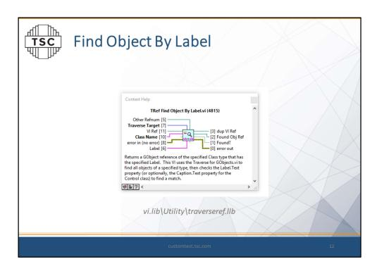
Tref Find Object By Label is an extremely useful VI that will get references to the objects on the front panel or the block diagram
